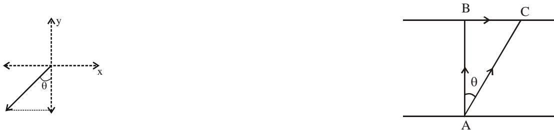
$\overline{AC}$  = Resultant velocity of boat = 10 km/hr
